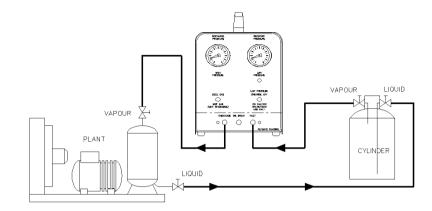
This method of recovery uses the unit to pressurize the refrigerant in the plant so that it can be discharged directly to a suitable recovery cylinder. This method is best suited to applications where more than 3kg of refrigerant is to be recovered.
