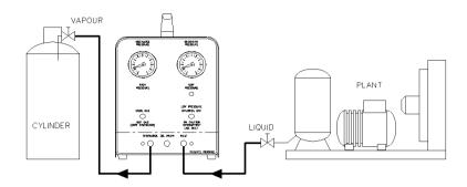
This method of recovery uses the unit to pull the refrigerant from the plant and discharge it direct to a suitable recovery cylinder. This method is best suited to applications where up to 3kg of refrigerant is to be recovered.
